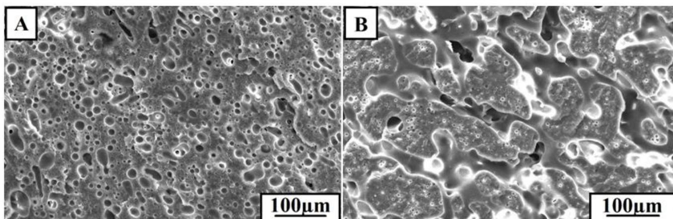
**Figure 1:** SEM images of impact fracture surfaces for (A) PPO/PA6 and (B) PP/PA6/PPO-g-MAH blends
