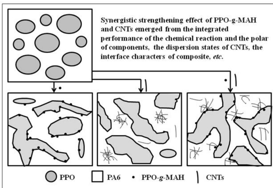
Figure 6: The synergistic strengthening effect of PPO-g-MAH and CNTs in PPO/PA6 blend
