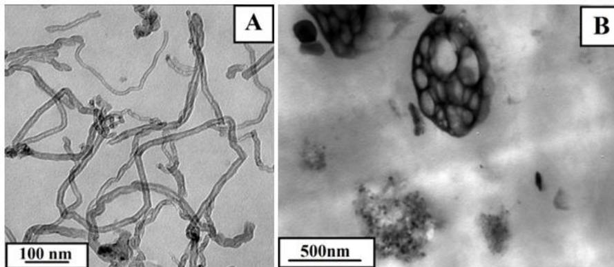
Figure 2: TEM images of (A) CNTs and (B) PPO/PA6/CNTs Composites
