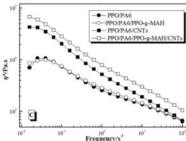
Figure 5: (A)  $G'$ , (B)  $G''$  and (C)  $\eta^*$  of PPO/PA6, PP/PA6/PPO-g-MAH, PPO/PA6/CNTs and PPO/PA6/PPO-g-MAH/CNTs composites
