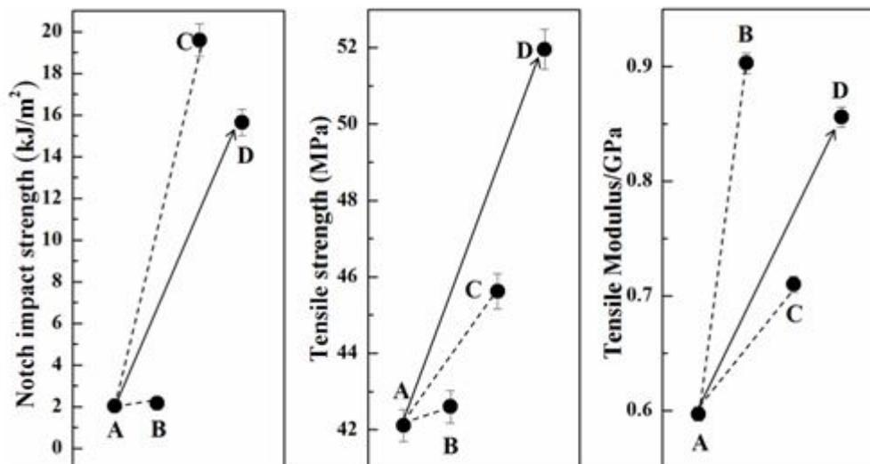
Figure 4: Mechanical properties of (A) PPO/PA6, (B) PPO/PA6/CNTs, (C) PPO/PA6/PPO-g-MAH and (D) PPO/PA6/PPO-g-MAH/CNTs composites
