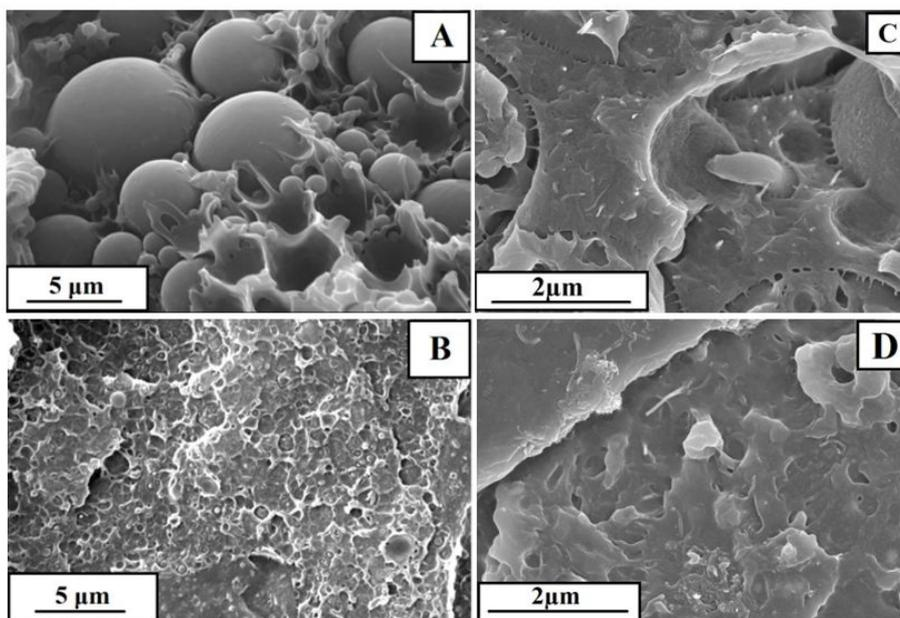
Figure 3: SEM images of impact fracture surfaces for (A) PPO/PA6, (B) PPO/PA6/PPO-g-MAH, (C) PPO/PA6/CNTs and (D) PPO/PA6/PPO-g-MAH/CNTs composites [6]
