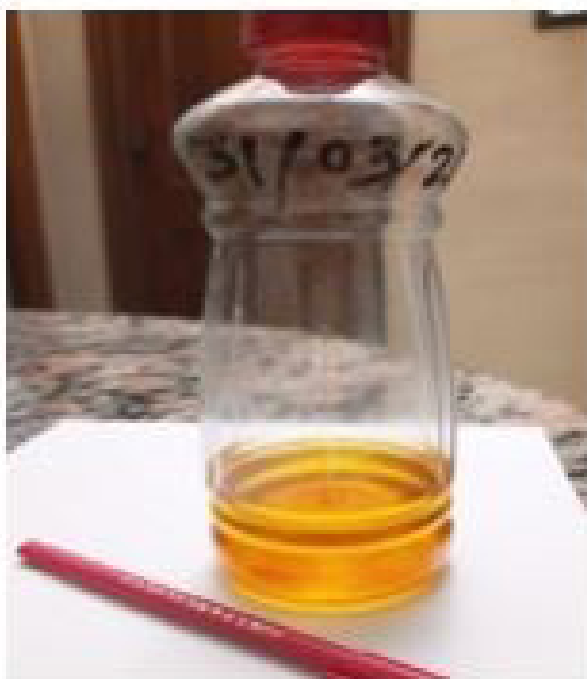
Figure 3: Fuel from Waste LDPE Plastic by Thermolysis Process
