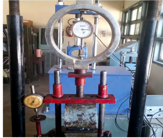
(b): Marshall loading head
