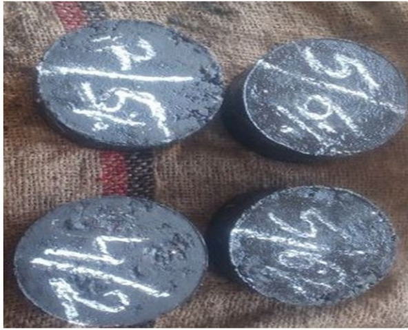
Figure 1(a): Marshall Samples
