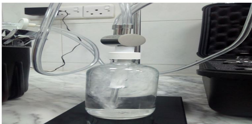
Figure 2: Aeration stage during radon measurement in tap water
